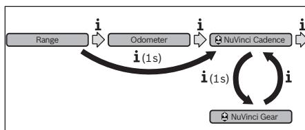
In the **<Gear Control>** mode, you can use the - or + button on the operating unit to switch back and forth between multiple defined transmission ratios. The engaged gear is shown on the display.
